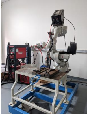
Keyhole TIG welding with a robotic arm
